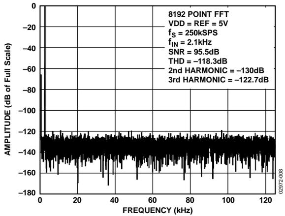
Figure 8. FFT Plot, VDD = REF = 5 V
