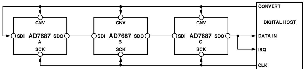
Figure 44. Chain Mode with BUSY Indicator Connection Diagram
