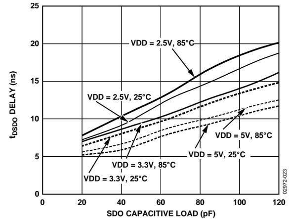
Figure 23.  $t_{DSDO}$  Delay vs. Capacitance Load and Supply
