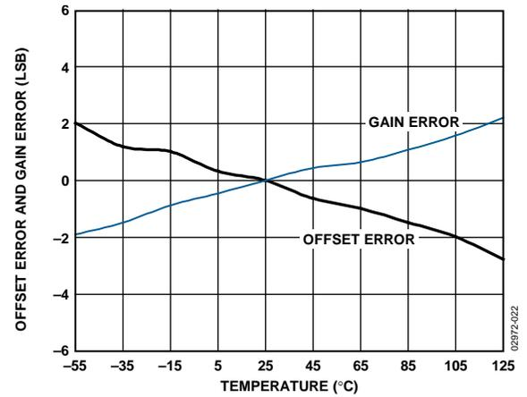
Figure 22. Offset Error and Gain Error vs. Temperature
