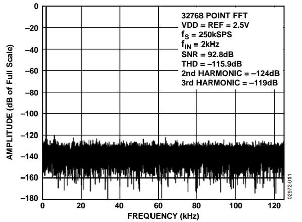
Figure 11. FFT Plot, VDD = REF = 2.5 V
