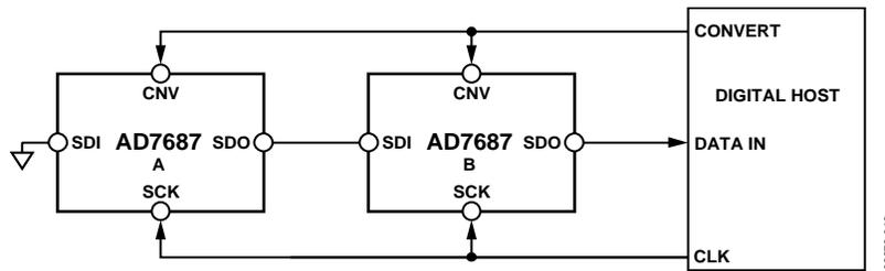
Figure 42. Chain Mode Without BUSY Indicator Connection Diagram
