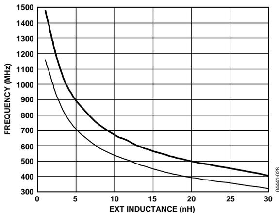
Figure 24. Output Center Frequency vs. External Inductor Value
