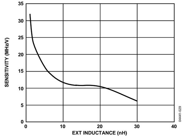
Figure 25. Tuning Sensitivity (in MHz/V) vs. Inductance (nH)
