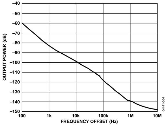
Figure 4. Open-Loop VCO Phase Noise, L1, L2 = 13 nH
