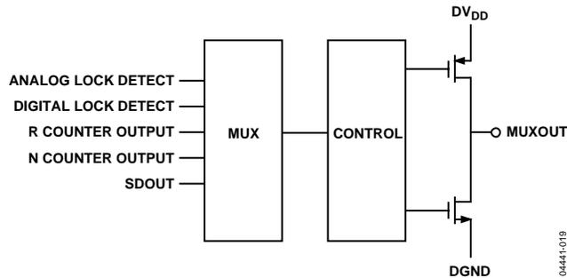
Figure 19. MUXOUT Circuit
