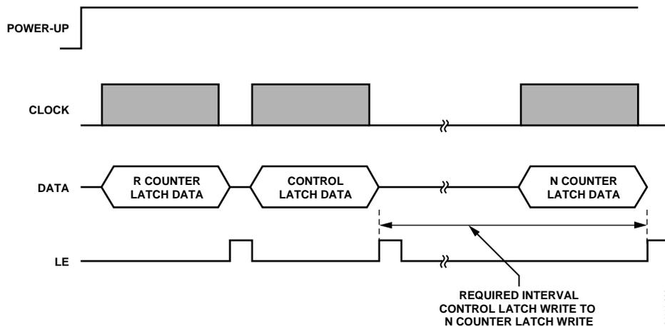
Figure 22. ADF4360-7 Power-Up Timing
