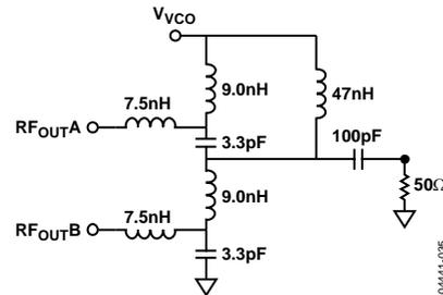
Figure 31. Balun for Combining ADF4360-7 RF Outputs
