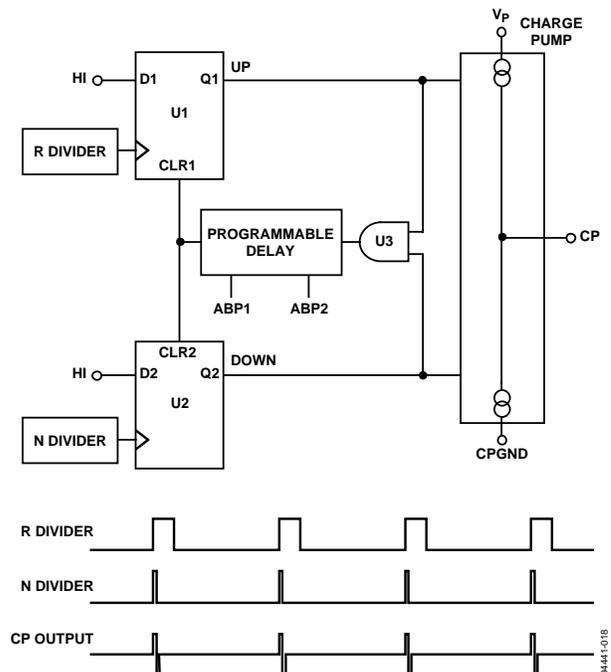
Figure 18. PFD Simplified Schematic and Timing (In Lock)
