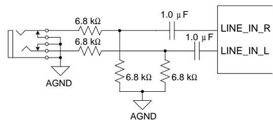
**Figure 18. Line Input (Replicate for Video and AUX)**
