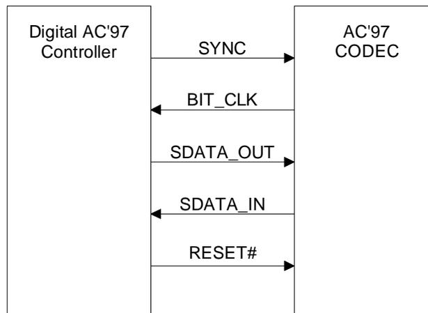
**Figure 7. AC-link Connections**
