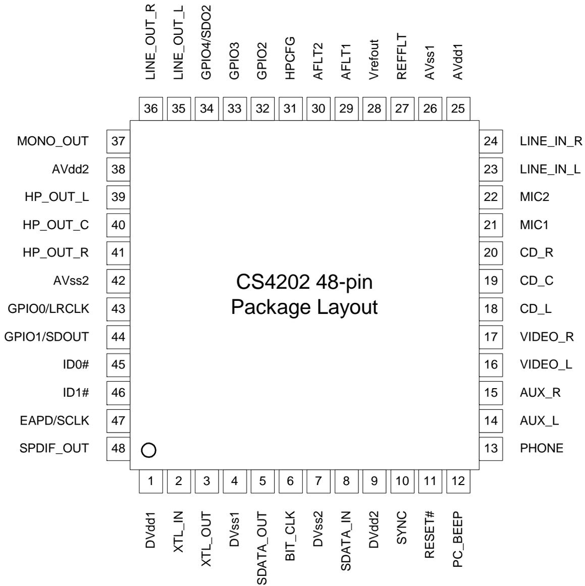
**Figure 27. Pin Locations for the CS4202**
