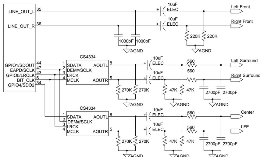
**Figure 10. Serial Data Port: Six Channel Circuit**
