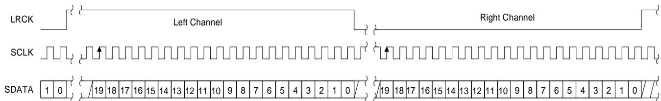
**Figure 13. Serial Data Format 2 (Right Justified, 20-bit data)**
