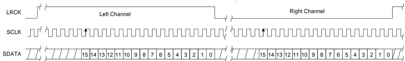
**Figure 14. Serial Data Format 3 (Right Justified, 16-bit data)**
