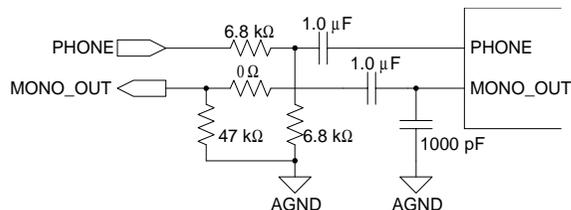
**Figure 22. Modem Connection**
