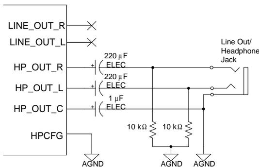
**Figure 24. Line Out/Headphone Out Setup**
