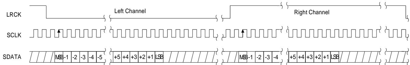
**Figure 11. Serial Data Format 0 (I<sup>2</sup>S)**
