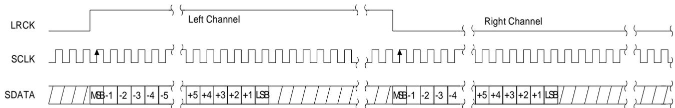
**Figure 12. Serial Data Format 1 (Left Justified)**
