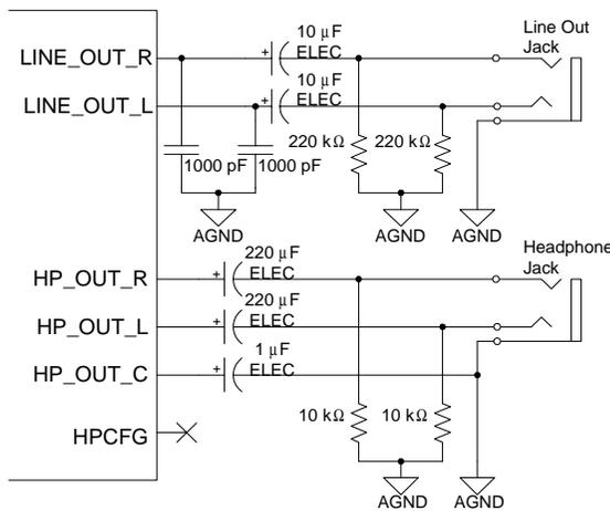
**Figure 23. Line Out and Headphone Out Setup**
