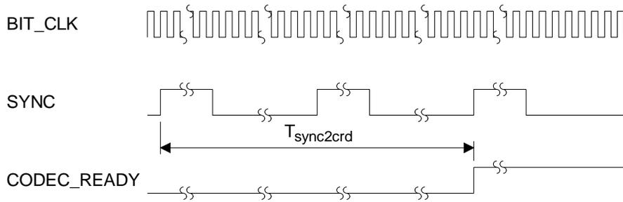
**Figure 2. Codec Ready from Start-up or Fault Condition**
