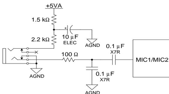
**Figure 20. Microphone Input**
