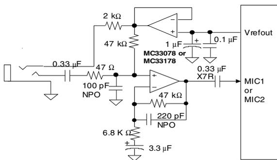
**Figure 13. Microphone Input**
