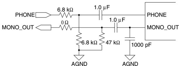
**Figure 16. Modem Connection**
