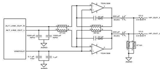
**Figure 18. Stereo Output**
