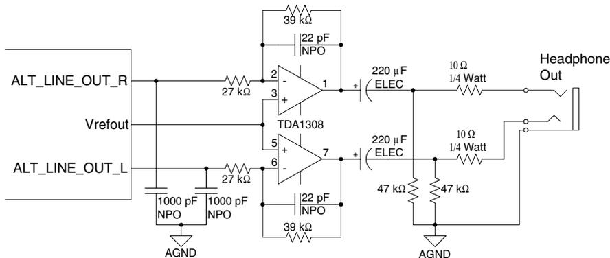
**Figure 17. Alternate Line Output as Headphone Output**
