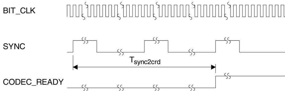
**Figure 2. Codec Ready from Startup or Fault Condition**
