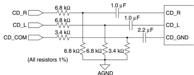
**Figure 11. Differential 2 V<sub>RMS</sub> CD Input**
