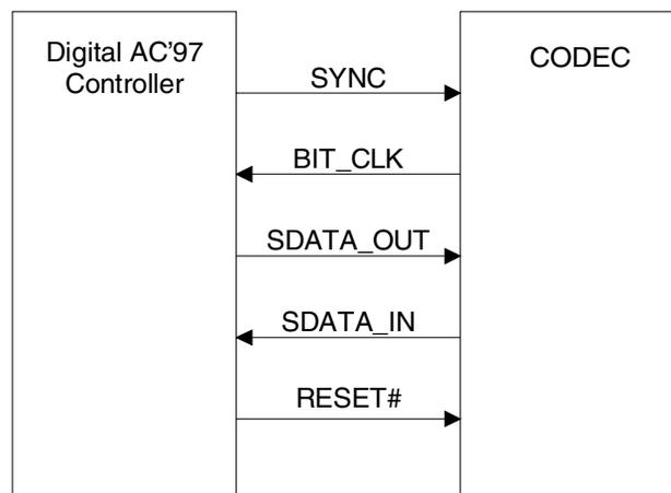
Figure 7. AC-link Connections
