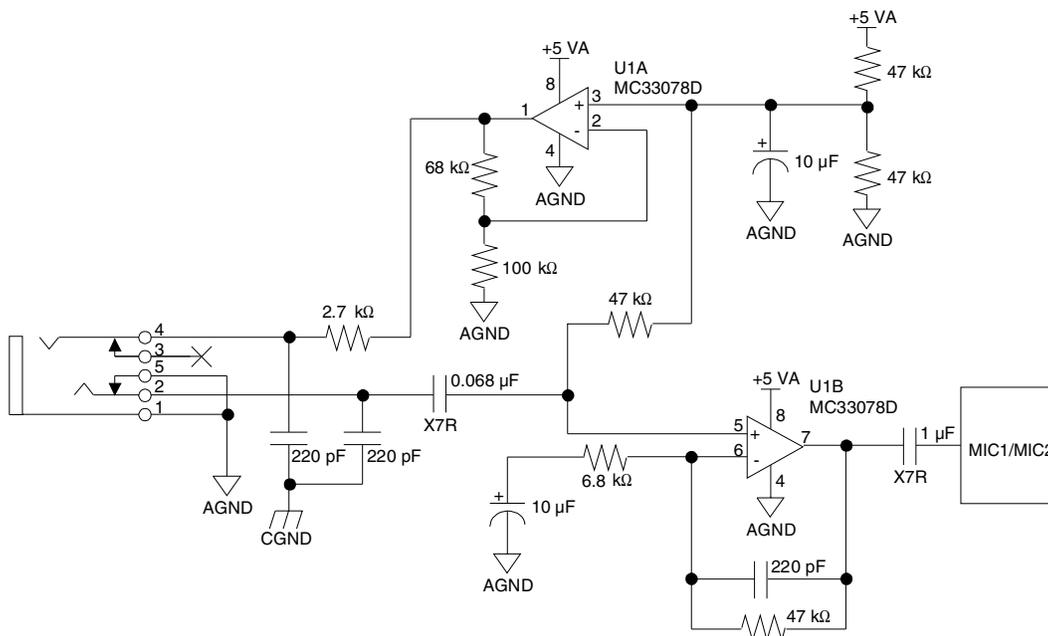
**Figure 14. Microphone Pre-amplifier**
