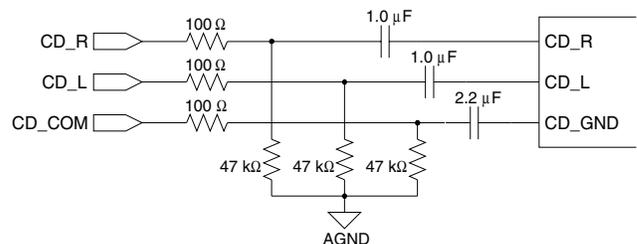
**Figure 12. Differential 1 V<sub>RMS</sub> CD Input**
