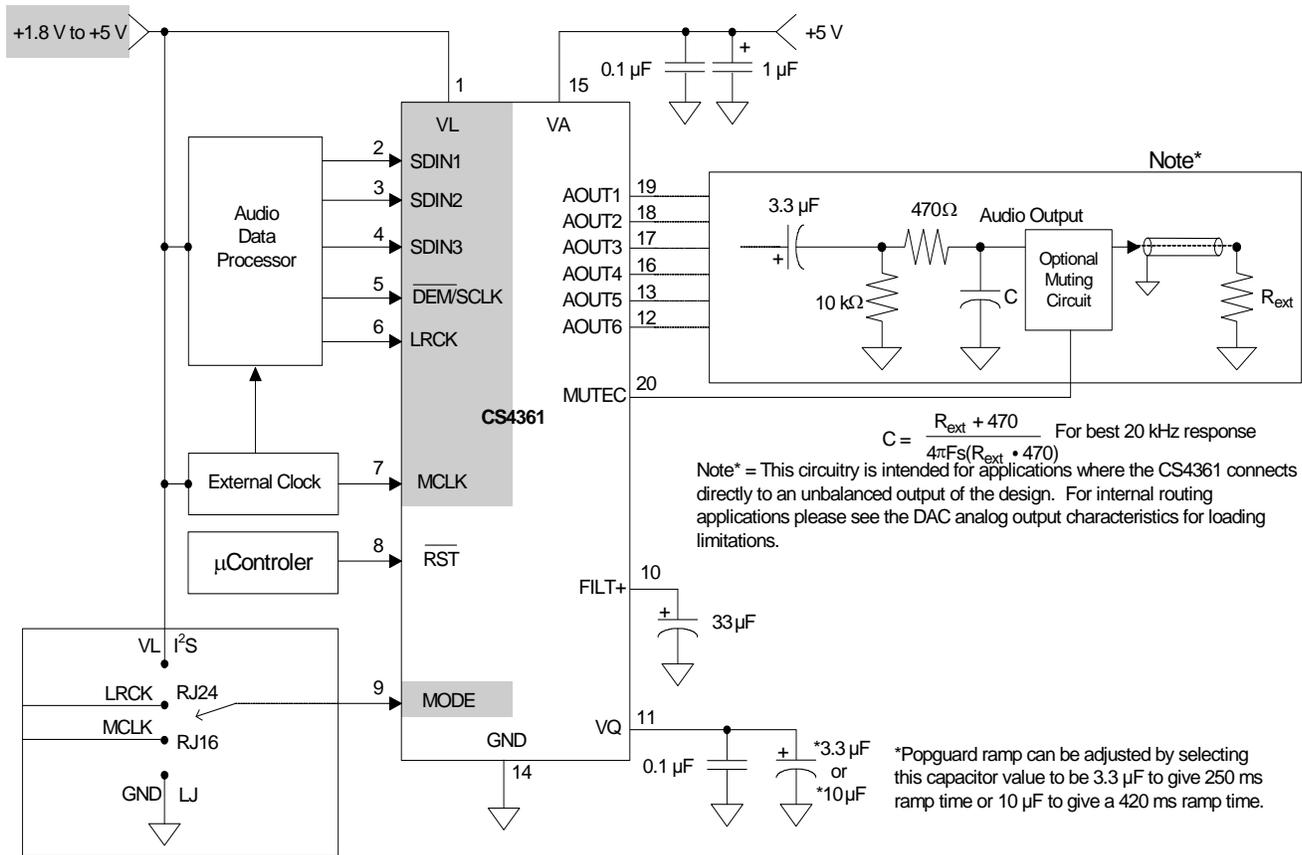
**Figure 6. Recommended Connection Diagram**
