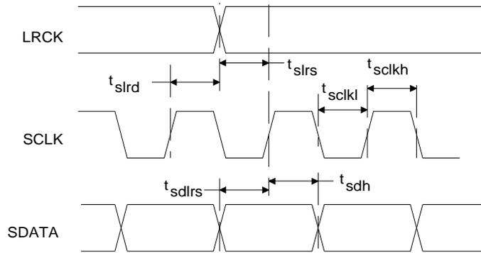
**Figure 3. External Serial Mode Input Timing**
