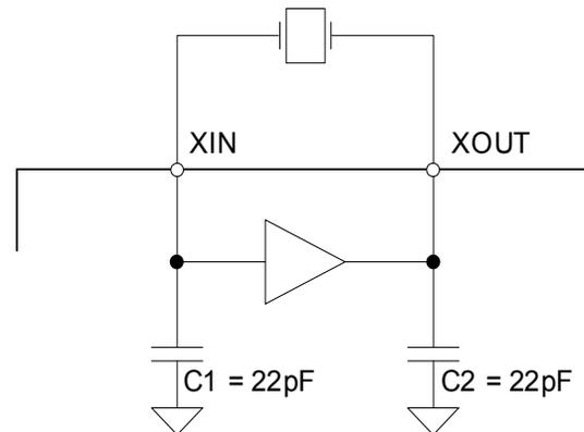
**Figure 1. Oscillator Connections**
