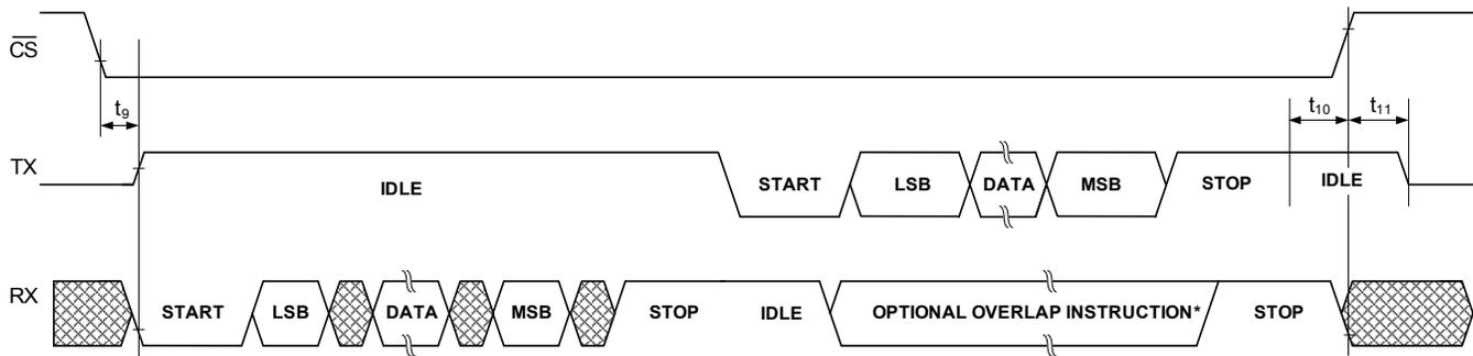
\* Reading registers during the optional overlap instruction requires the start to occur during the last byte transmitted by the part
