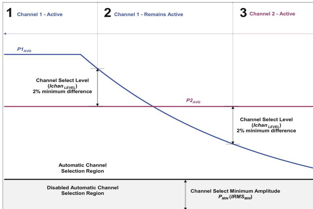
**Figure 15. Automatic Channel Selection**
