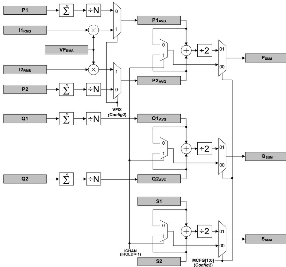
**Figure 14. Channel Selection and Tamper Protection Flow**
